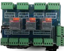
Fan Coil Multiplexing Board
