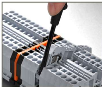
Removal of Terminal Blocks
